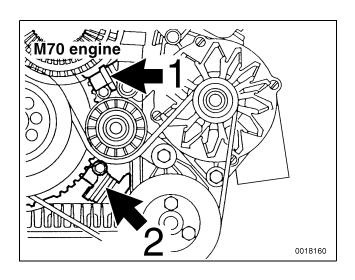
Crankshaft position/rpm sensors on M70 engine (arrows) mounted on front timing chain cover. Upper sensor is for DME 1, lower sensor is for DME 2.
