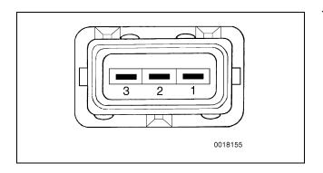
Using digital multimeter, check resistance between terminals 1 and 2 in crankshaft position/rpm sensor connector.
