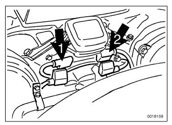
Disconnect crankshaft position/rpm sensor harness connectors on M70 engine for right bank (1) and left bank (2) of cylinders.
