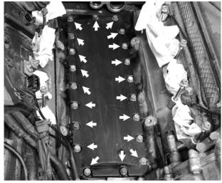
Remove bolts from valley pan (**arrows**) and remove pan. It may be necessary to pry up on front of pan to loosen.
