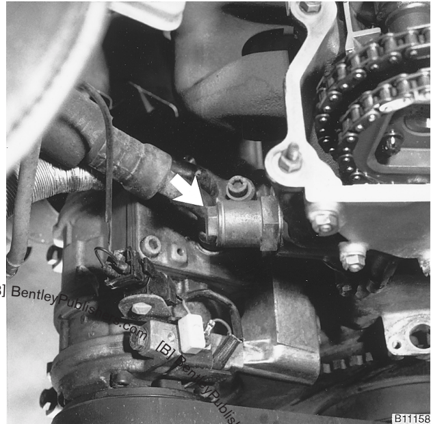
Fig. 40. Primary timing chain tensioner bar (arrow). Remove tensioner slowly to relieve spring tension beneath end plug.
