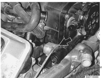
Remove tube locking clip (arrow) and slide vent tube forward.
