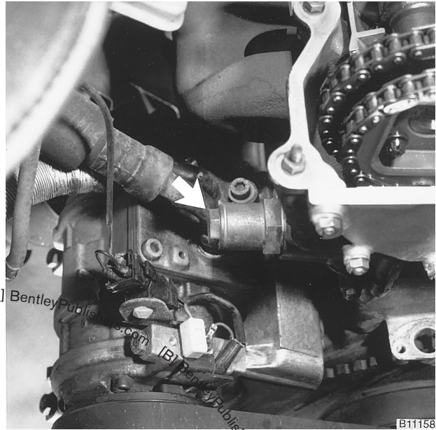
Fig. 37. Primary timing chain tensioner (arrow). Remove tensioner slowly to relieve spring tension beneath the end plug.
