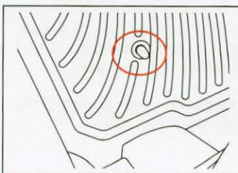
1. Make sure the driver's floor mat is properly secured by the retaining hooks (clips). Confirm that the retaining hooks (clips) are secured into the grommet holes in the vehicle's floor (carpet).
