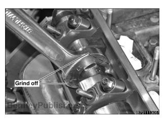
In procedure steps that follow, use 27 mm open-end wrench to counterhold each camshaft at hexagonal casting before loosening camshaft sprocket fastener. If necessary, grind off outer edges of wrench jaws to prevent damage to cylinder head.
