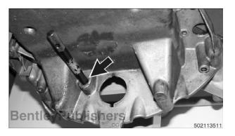
Lock crankshaft in TDC position with BMW special tool 11 2 300 (arrow).
