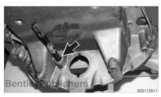
Lock crankshaft in TDC position with BMW special tool 11 2 300 (arrow).
