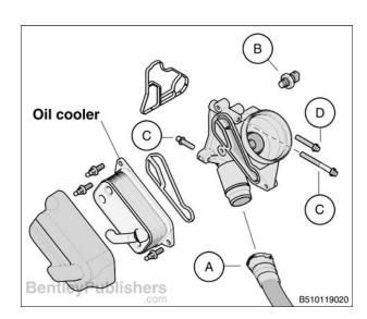
Oil filter housing, removing and installing (N54 engine)
