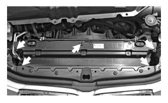
Remove Torx screws (arrows) from radiator cover and pull radiator cover up and off.
