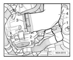
Remove intake hose - 4 - . To do so, disconnect air hoses - 1 - , if present, and - 2 - (compress securing ring) and remove spring clamp - 3 - .
