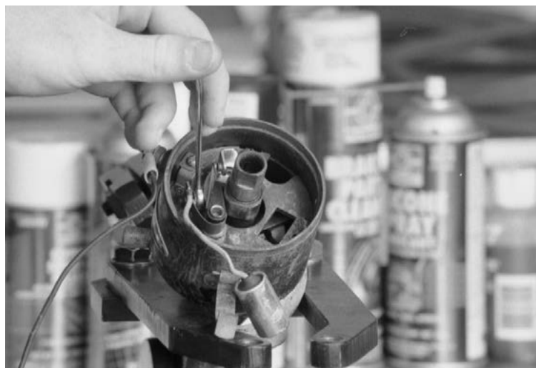
On the bench, the condenser and points come out easily. Old Autolite point sets have one hold-down screw. The breaker arm pivot slides over a support pin on the breaker plate.
