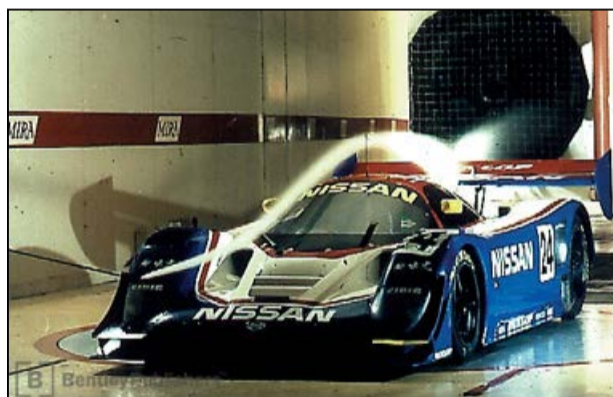
Use of smoke trace for off-body flow visualization in the wind tunnel test section.
