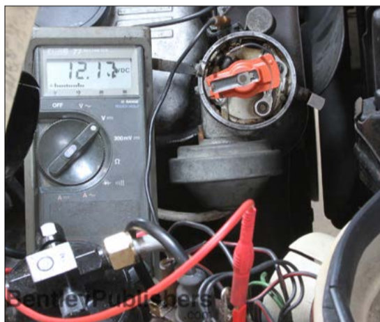
Setting static timing with a multimeter. (Chapter 5, "Setting Ignition Timing")
