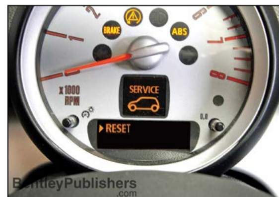
020 Maintenance Step-by-step instructions on resetting CBS service items.
