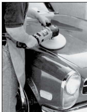
Chapter 9, How to Wax Your Car Like the Pros Polishing with a fine cleaner to remove paint scratches.
