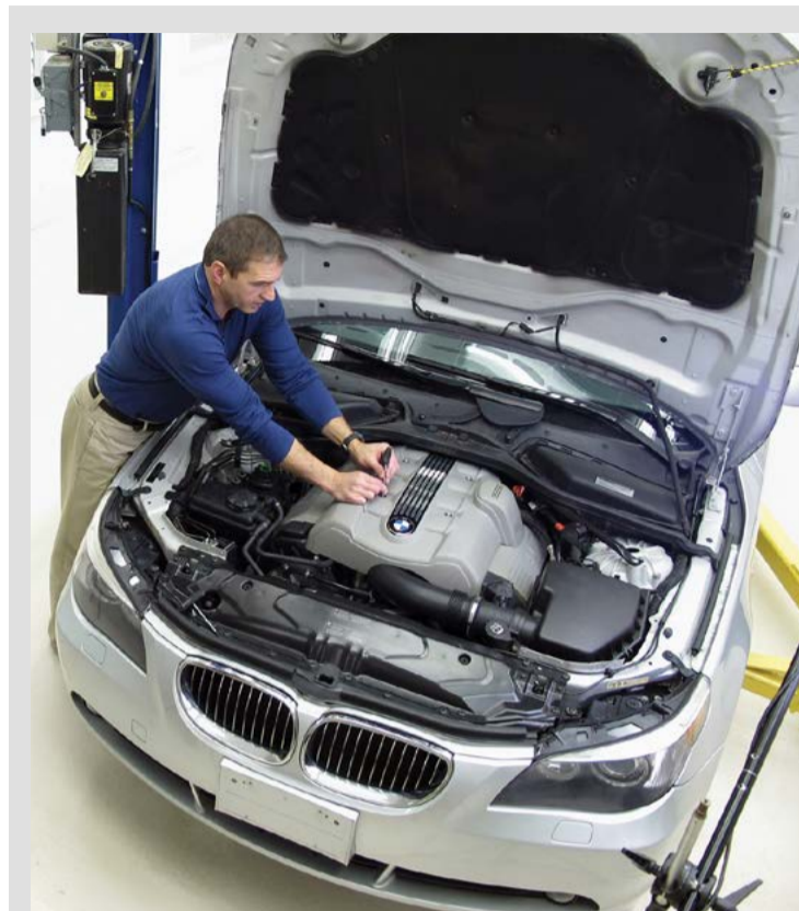
Bentley technical editors removing motor cover on V8 (N62) engine.
